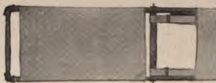
FIG. 362.—Gas-pipe bed tray, covered with sections of canvas for cleansing. (Bradford)
